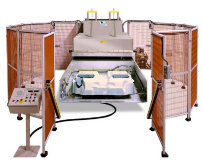
For the welding of reinforcements on thermoformed car carpets
