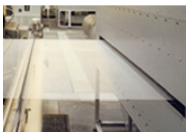
Bimodular radio-frequency tunnel for high-speed drying of textile yarns, after textile sizing, on stretching-glueing lines
