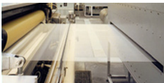
Bimodular radio-frequency tunnel for glue and resin drying, for dipping on large title yarns and cords
