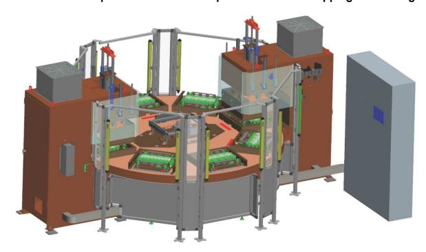
For the production of flexible type blood filter in PVC film
