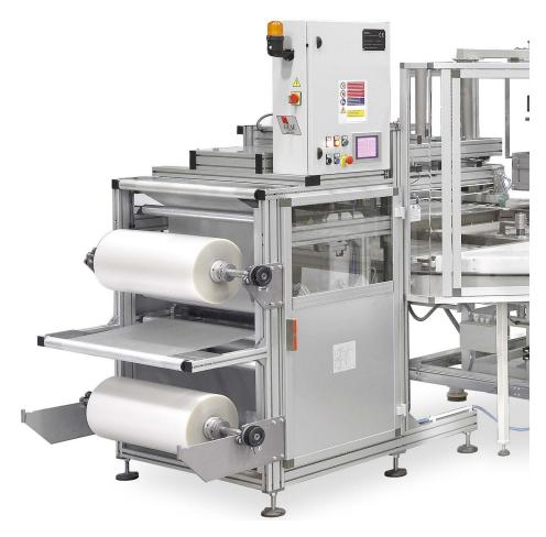
For the automatic loading of 1 or 2 PVC sheets, from reel, on the turntable stations
