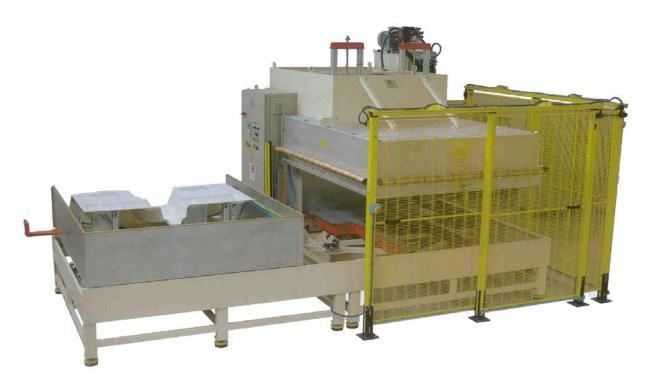
For the welding of reinforcements on thermoformed carpets
