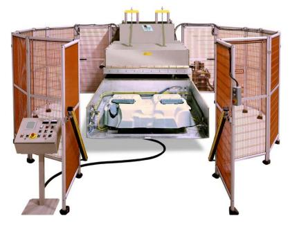
For the welding of reinforcements on thermoformed car carpets
