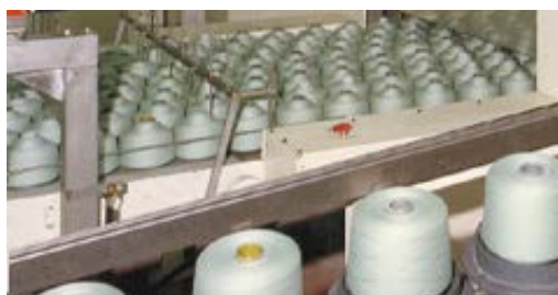
Tunnel for radio frequency drying of textiles yarns, hanks, tops e tights, after dyeing
