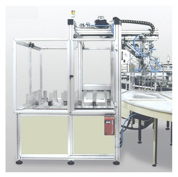
For the autoamatic loading of pre-cut sheets or pre-cut cardboards, on the turntable stations
